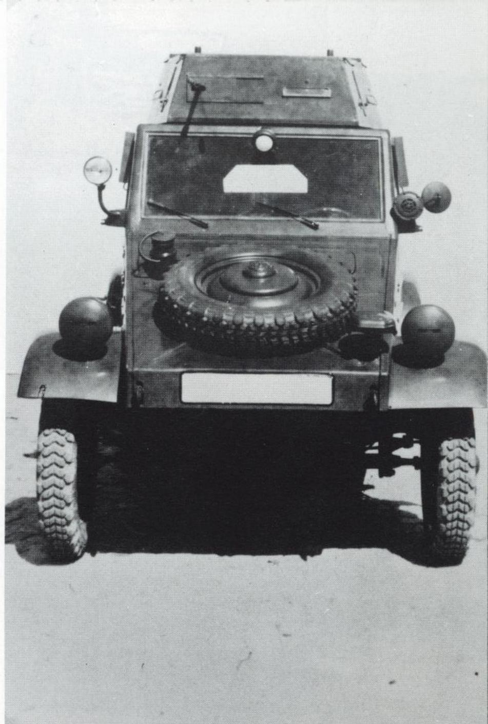
Right: Type 823 armored car mockup with machine gun turret, without road-wheel covering. Photographed May 17, 1941.
